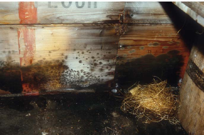
Fig. 2. Crates in galley area inside Cape Evans Hut affected by surface fungal growth. Fungi from samples of interior and exterior woods and artifacts from the historic huts were used in this study to compare to fungi obtained from soils.
